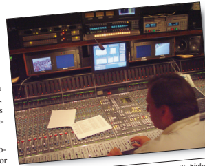
Figure 2.12 High-end production trucks come with high-end audio mixing consoles that are often married to a computer (the center screen is a GUI for setting up the audio console). These complex mixers allow for detailed processing of each audio source, and the audio processing of each source is often convoluted of paths, taking audio sources through the console multiple times as sources are sub-mixed and then finally mixed into a composite audio signal.
