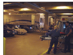
Figure 2.14 Often the truck must be parked inside the venue, in which case the path to where it will park must be navigable. There were a couple of well-known venues where the ramp the trucks had to traverse was too steep, causing some trailers to touch ground, or beach, when the tractor started down them. Often the clearance between trailer and ground is less than a foot. It is also helpful to know what will surround the truck at game time. The two production trailers shown are surrounded by emergency crews and the expensive cars of professional hockey players as the event start time draws near.
