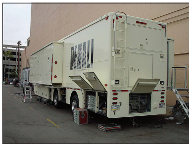
Figure 2.13 Above: Trailer parking can be simple, as is the case here, or there may be lots of obstacles involved. The survey must identify where power for the truck will be obtained, and determine that enough space exists that the truck and its equipment bays will be accessible.
