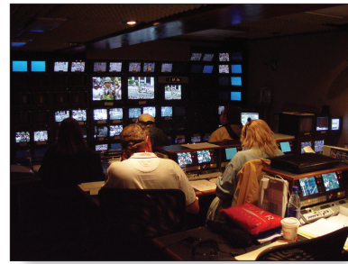
Figure 2.11 Production compartment in large remote truck covering a parade. The TD is the second from the right. The rest of the crew members shown are directors, producers and their assistants. In a live production such as this, one of these people will be in contact with the people assembling and releasing parade participants to synchronize the parade and the televising of it. Another person will be in contact with the television station(s) to synchronize the commercial breaks with the parade.
