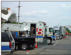
Figure 2.10 For the Indianapolis 500 the local station providing coverage for itself and other stations across the country used a vendor's remote truck for the production, but its own Ku satellite uplink truck to get the signal back to its own and other stations. This link from venue to broadcast facility is known in the industry as the backhaul.
