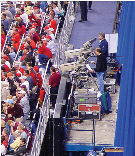
Figure 2.18 Places that don't normally see television cameras, such as a parade, will definitely need temporary camera platforms.
